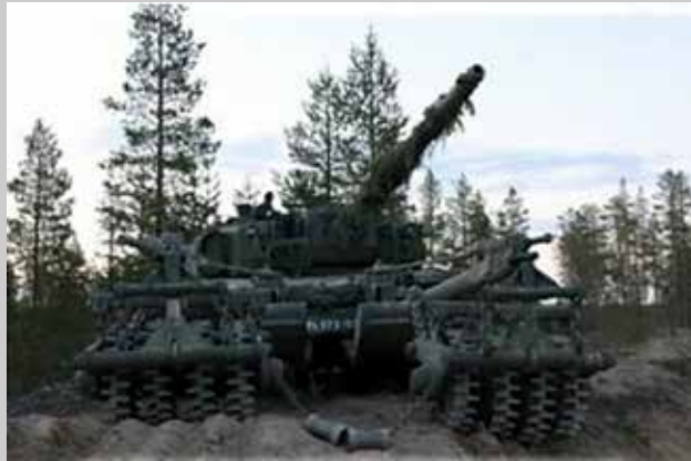
Figura N° 11: MCRS (Mine clearing roller system).
